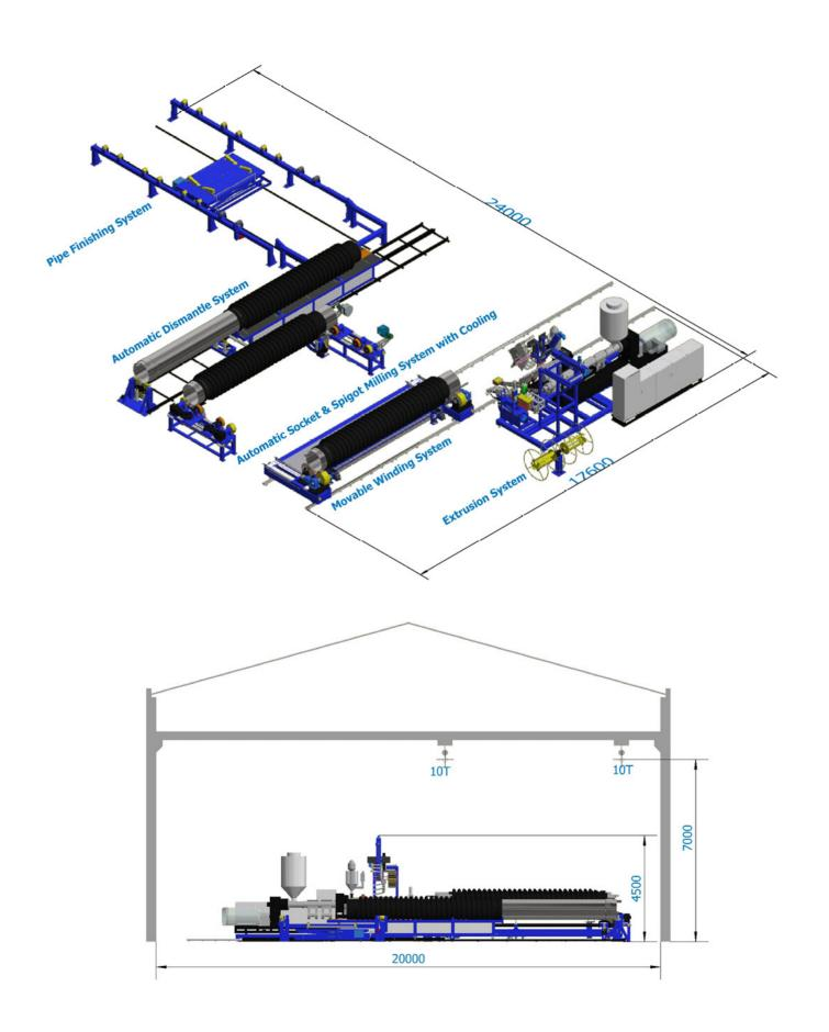
The extrusion system consists high efficiency extruders, computer control system, dual color inner wall die and outer coating layer die, melt distribution valve, pressing and guiding unit, co-tube feeding unit, gas heating system and infrared heating system
